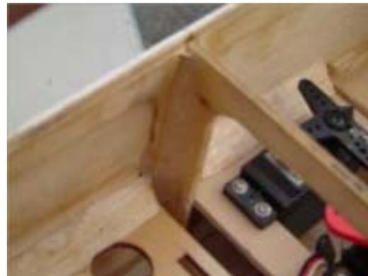
The firewall was attached last to have easy access to the gear plate and fuel compartment so those areas could be reinforced before the last gluing.
