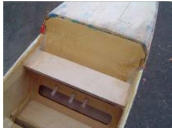
The battery/receiver plate re-attached, the bulkheads are glued and strengthened by the use of fillets made with the non-sag Epo-Grip #30 Paste making the task easy.
