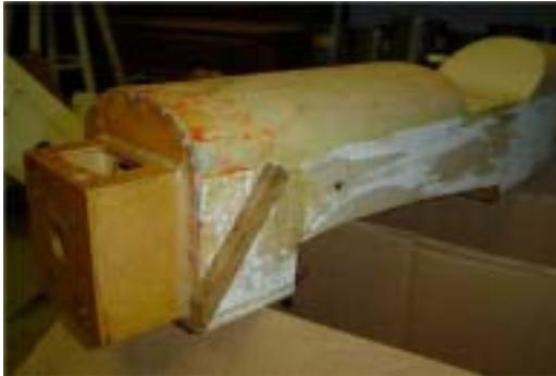
Once the firewall was attached and all the repairs completed the fuselage was filled and sanded smooth removing most scars before covering.
