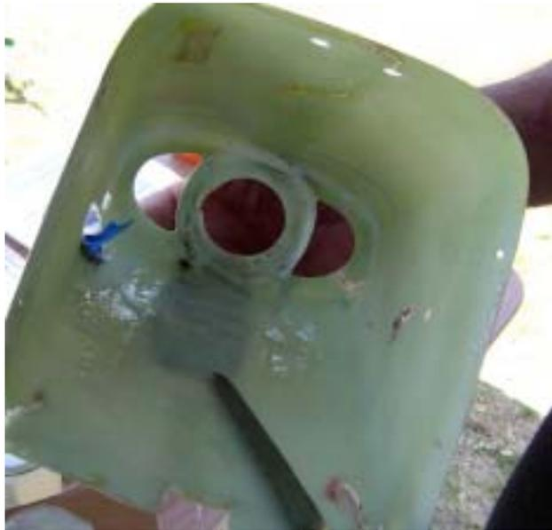
After you have the cowling openings replaced to your satisfaction its time to sand and prime making the cowl ready for paint. Use auto body glazing putty for removing any final flaws before final priming and paint.
