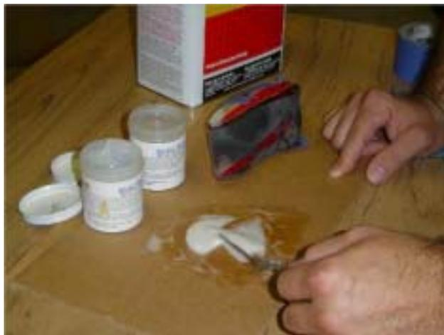
Next apply a thin layer of material on the inside of the canopy. It may take you more than one mixing to reinforce the canopy for the repair. In roughly 5-7 minutes you will feel the heat of the
