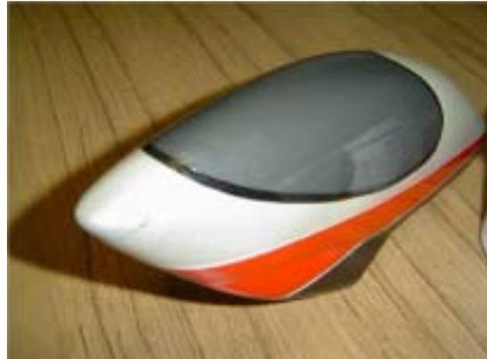
In the repair of a fiberglass canopy, the same process is used. However, in the end you will need auto body glazing compound to fill in areas where the gel coat has cracked away on the outside of the canopy. Just over fill those areas with the putty and allow the material to dry. Once the material is dry, wet sand the putty smooth, then paint the damaged areas.
