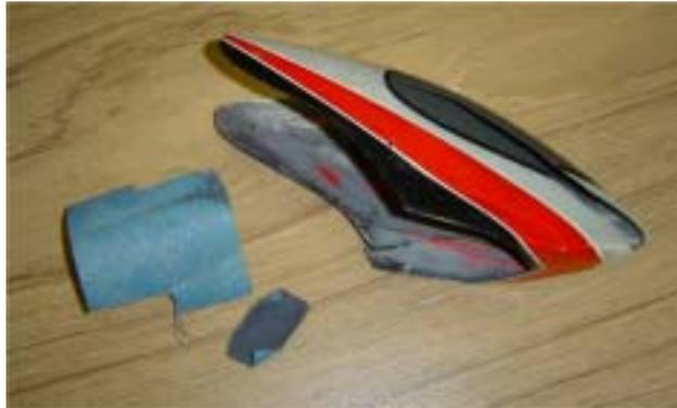
Next on the outside take the painters blue masking tape and tape the canopy back together. Take care in this procedure and only a fine crack is left to touch up. Once the canopy is taped together, wipe the interior with the Denatured alcohol to remove any oils left by fuel or fingerprints.
