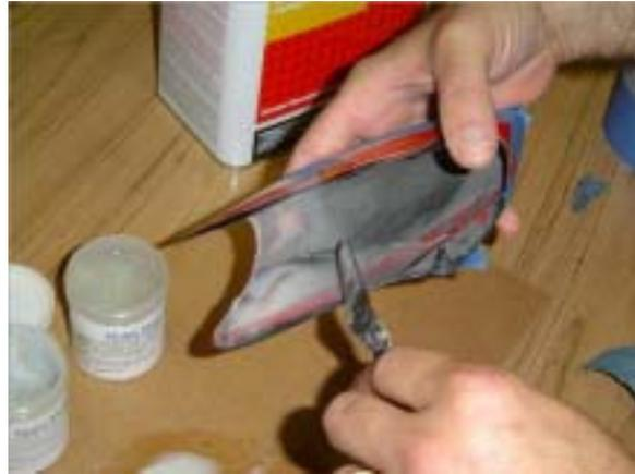
Once you have good coverage in the areas to be repaired inside you canopy let the material cure for another 20 minutes. After the time has elapsed remove the tape from the outside of the canopy. The canopy is now repaired and ready for paint.
