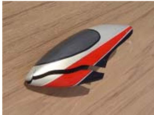
The supplies needed to repair this ABS canopy are nothing out of the ordinary and can be easily obtained. All that is needed is Denatured Alcohol, sand paper, painters blue masking tape, Epo-Grip Model Matrix, a mixing surface, and a mixing knife or popsicle stick.
