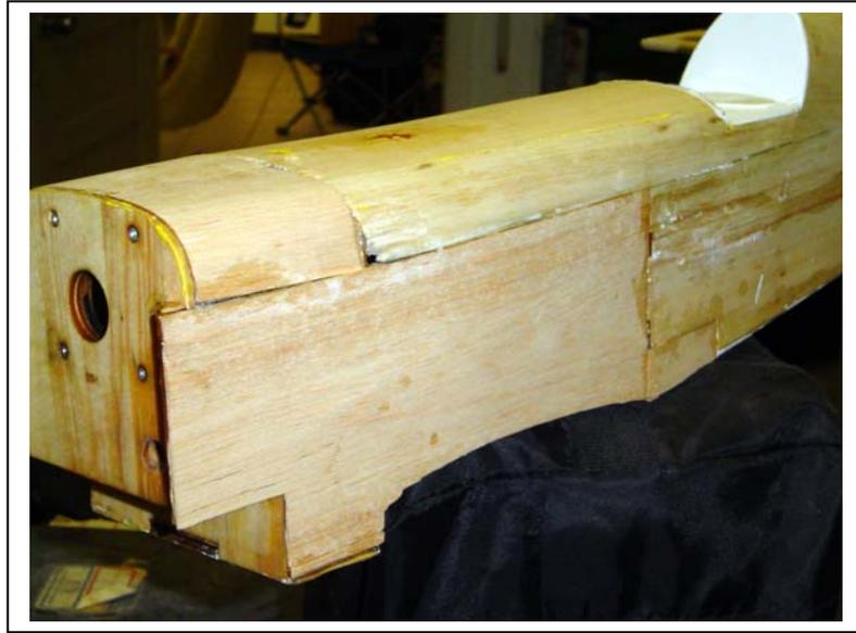
Once filling and final sanding are completed you are ready to cover the airplane with your own color scheme. The wings on this airplane were in pretty good condition, only requiring some minor rib and wing tip repairs. We will cover wing repairs in another section.
