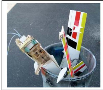
The first step of the rebuild process is to strip off all covering from the airplane and clean all the parts. This allows you to carefully examine the airframe looking for damaged areas. It also lets you take inventory of the parts, what has to be fabricated, and make notes where repairs have to be accomplished.
